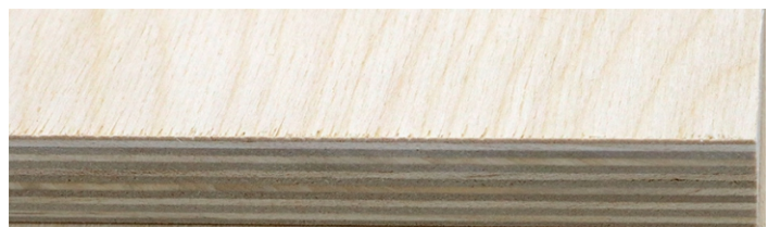
Baltic Birch Plywood has 13 plys
